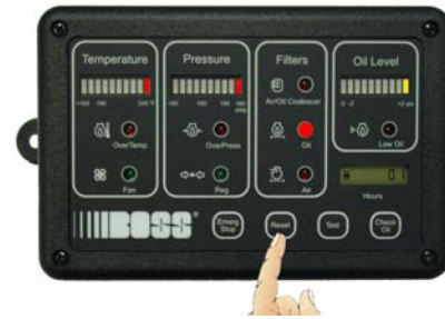
Step 3. Oil In-Service will reset to 0
